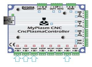
Sensors/switches Home for the **X**, **Y** axis can be mounted on either side of the axis (for zero or maximum points).
