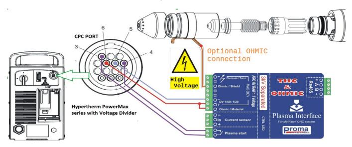
WARNING !!!! A high voltage may occur on the OHMIC SHIELD cable of the touch system (see the documentation of the plasma cutter) - use a cable with appropriate / double insulation.
