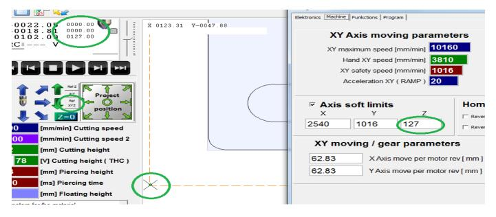
A reference base/reference drive with program limits is not required for machine operation. However, it allows precise determination of the position of axes within the machine and easy return to interrupted operation, e.g. after a power outage or other failure.
