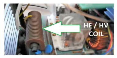
In order to minimize the interference generated by cheap/Chinese plasma cutters, it is recommended to connect the measuring wire before the coil (transformer) of the HF/HV ionizer. Most often it is the first element connected directly to the air/current connection of the plasma torch.
