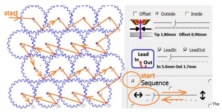
**MyMiniCAM** module is very simple and has only the basic necessary functions to automatically, very quickly and conveniently generate tracks from the drawing. **For more demanding projects use any external CAM program.**
