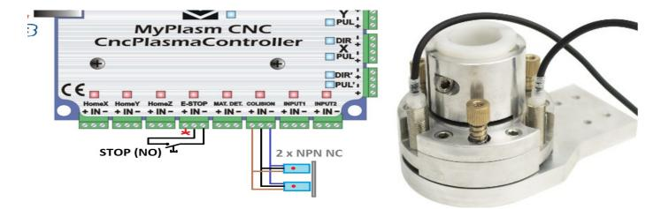
In the example, a combination of two **NPN NC** sensors is used, which in normal operation have continuous contact with metal and thus do not give a signal, in case of a torch collision with the material, the sensor is activated and the collision stop is activated.
