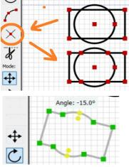
In addition to the basic drawing tools, the program has an intersection detection function, which makes it very easy to create resulting objects after removing unnecessary lines with the scissor tool. (delete).
