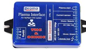
Plasma Start - relay contacts switching the plasma Current sensor - not connected ! ( option withdrawn )
