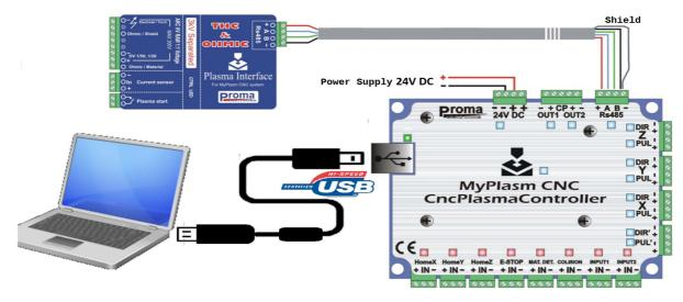
After establishing the communication, the compatibility of the controller's firmware version with the program version on the computer will be checked and, if necessary, the firmware in the controller will be updated.
