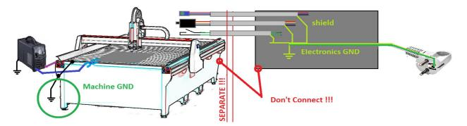
MyPlasm CNC system works with any plasma source, but cheap / Chinese sources with HV / HF ionizers generate very high EMC interferences, so when the arc is glowing or fading, problems such as mouse suspension, keyboards, monitor dimming, computer reset and various other operating interferences can sometimes appear. The impact of interference can be minimized to a large extent by moving the torch cable and plasma source away from the automation system.
