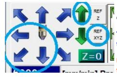
Lift the Z-axis upwards, the X-axis upwards to the Left and the Y-axis downwards (to yourself) and click REF XYZ.
