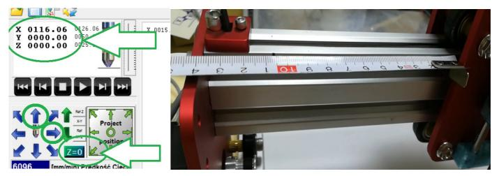
Tip: According to MyPlasm CNC users, the best results (high dynamics, speed and precision) are obtained with identical X,Y axis ratios within the range of 30-80mm feed rate per motor revolution and 8-20mm per motor revolution for the Z axis.
