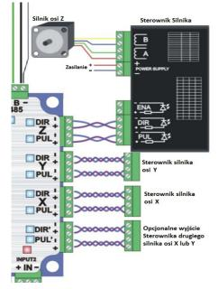
The MyPlasm CNC controller has **PUL/DIR ( Step/Dir )** outputs to control 4 stepper motors, servo-steppermotors or servo drives. In order to minimize the impact of interference on the control signals, the connections should be made with twisted pairs of wires as shown in the figure.
