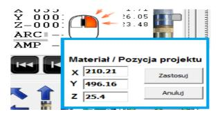
In the same Coordinate Edit window can be used to edit the torch position relative to the material which will move the project relative to the current torch position :
