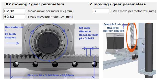
For the Z axis, this is usually the pitch of the drive screw thread, taking into account possible gear ratios.
