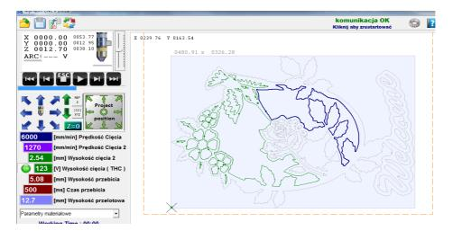
You can also point to an object with the Right Mouse button in the preview window, in addition, it is possible to indicate the location of the path from which it is to be executed:
