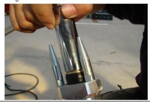
9. Rotate the gun tail pressure regulator to moderate pressure, lock tight.
