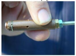
7. When the collet is inserted into the core, the tip of the stud needs to be higher than the vertical plane 2-3mm.
