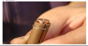
6. Insert the fitting stud collet that will weld.
