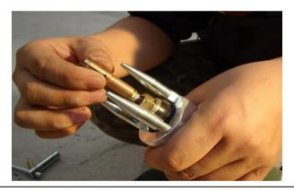
8. After loading the stud collet, turn the sleeve clockwise to tighten the lock.
