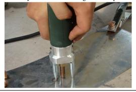
16. Welding is done, visual inspection, and an iron hammer is used to bend the study to 30 degrees.
