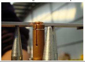
2. Insert the switch line of the welding gun into the air joint and tighten the lock nut.
