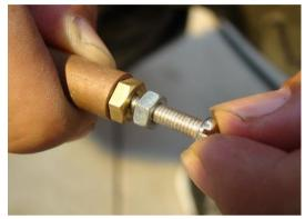
5. When the adjustment is completed, tighten the retaining nut at the end of the clamping head.
