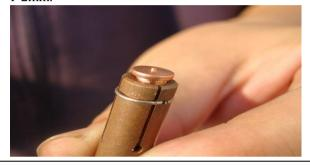
6. Insert the fitting stud collet that will weld.
