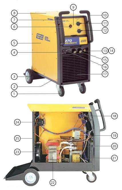
Fig 8 Weldmatic 270 Power Source Assembly
