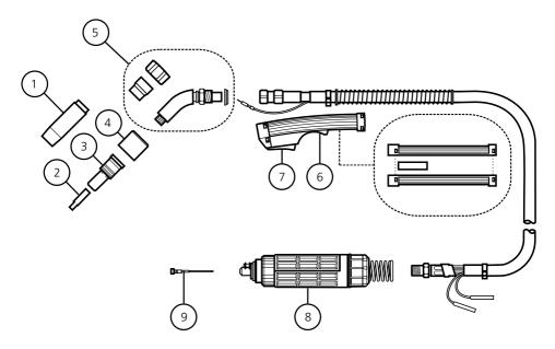
Fig 9 GUN001 (200 amp) Gun and Cable Assembly
