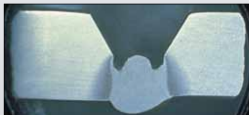
Open Root Pass with Stick Electrode
