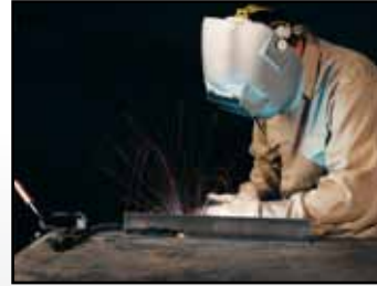
STT® using CO 2 and .045 in. solid wire. Note reduced spatter and fume.
