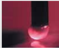
Conventional CV short circuit transfer using CO 2 and .045 in. solid wire.
