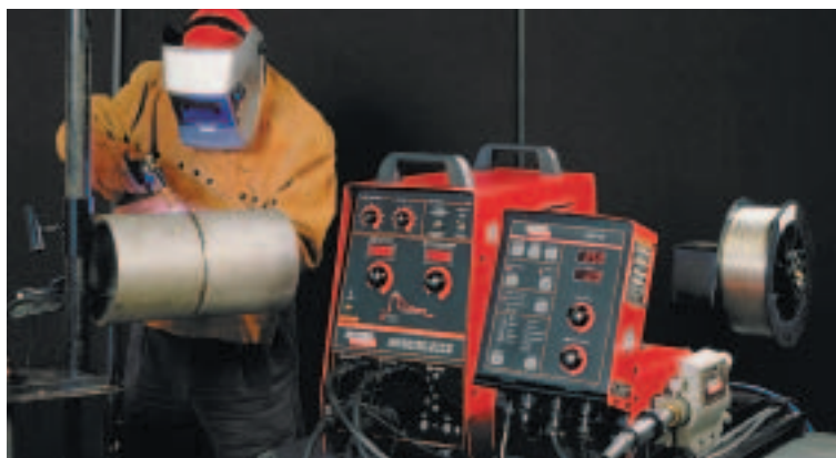
STT process using 100% CO 2 and .045 in. (1.2mm) wire.
