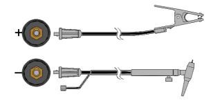
Connect the torch cable to the (-) terminal of the machine and the work clamp to the (+) terminal. Insert the connector with the key lining up with the keyway and rotate approximately ¼ turn clockwise. Do not over tighten. Finally, connect the gas hose to the gas regulator on the cylinder of gas to be used.
