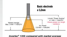
Amps are not the only requirement! A good start and smooth arc requires more than simply amps and voltage. The Invertec<sup>®</sup> range is equipped with POWER SURPLUS in addition to normal welding current. This advanced control monitors the arc, constantly adjusting output to ensure a stable arc and first-rate starting, even when the arc-lenght varies greatly.
