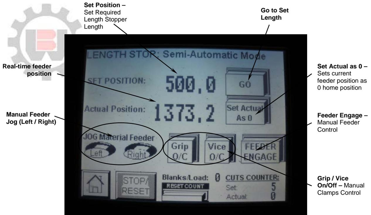
Figure 3.11 – Length Stopper Control Screen
