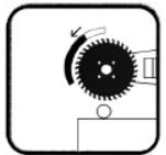
**Do not attempt to operate the machine unless all safety guards are in operation.** The guard must fully cover the blade when the head is in the uppermost position.
