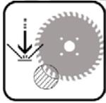
**If the blade becomes jammed, stop the saw immediately.** Use manual jog backward to release the specimen.
