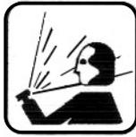
**Any maintenance work performed on the hydraulic, pneumatic or coolant systems must be carried out only after the pressure in the system has been released.**
