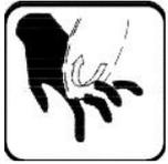
**The Operator must not conduct any risky operations** or those not required in the course of normal cutting (e.g. remove swarf from the machine while cutting).
