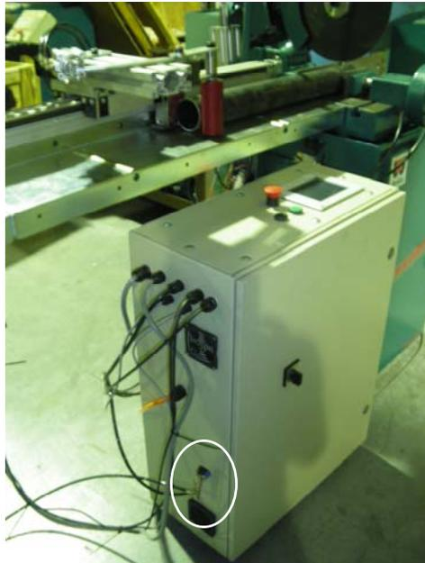
Figure 3.1 – Main Air-Supply Connection
