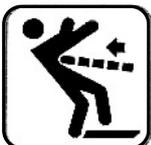
**Do not wear oversize clothing** with long sleeves, oversize gloves, bracelets, necklaces or any other loose object that may become entangled in the machine's blade during cutting. Long hair must be tied back or placed in a hair net.
