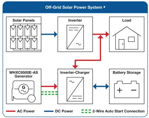
♦ Depending on system configuration, the generator can automatically provide backup to recharge the storage battery and / or feed in power to supply the load.
