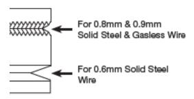
\*Knurled groove is suitable for both Solid & Flux-cored (gasless) wires in this machine.
