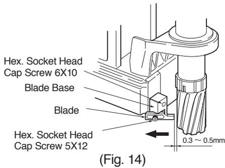
Chip Breaker is to shred down cutting chips in randomly short length that are produced during the drilling operation for easy discharge of the succeeding cutting chips.
