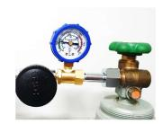
Then, open the purge valve. After doing that open the needle valve slowly allowing a small amount of CO₂ to vent through the purge valve. You will know it is venting as a white vapour will be released.
