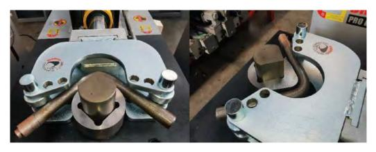
Shown here is 32mm mild steel round bar bent to  $90^{\circ}$ . Mild steel up to 32mm may be bent using the small radius (except rebar for structural use).
