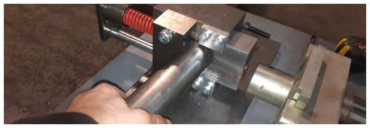
Offer the end of tube or pipe over the punch and move ram forward until crop is completed. Retract ram.
