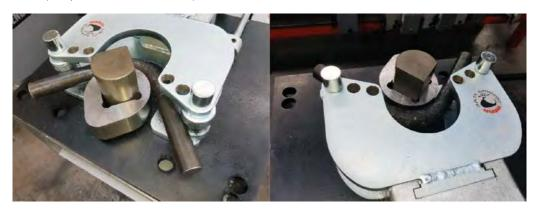
Shown here is 32mm rebar bent to  $90^{\circ}$  (note orientation of former and placement of roller pins).
