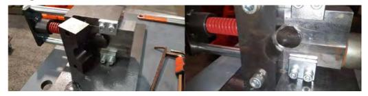
Using the 2 x m12 cap screws secure the die in place. Tool is now ready to use.
