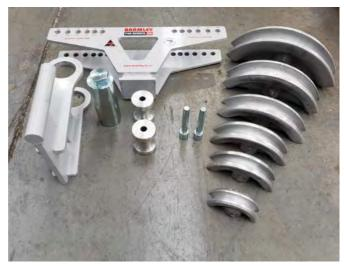
• The first step is to retract Hydraulic Ram and turn hydraulic system off. Remove any tooling from the Hydraulic Ram and slide the Frame into the tee slot on the end of the Hydraulic Ram. This holds the Frame securely onto the end of the Hydraulic Ram.
