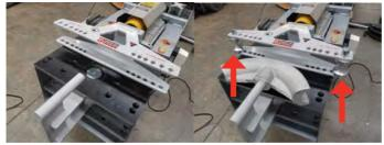
• Move Control Lever forward to bend pipe to desired angle (inching can be done easily). If multiple bends are required, before retracting ram and while ram control lever is in center position (neutral), move Stop as far left as possible and tighten (some re-positioning may be required to find exact stop location). This will push control lever in to center position (neutral) to allow consistent bends when correct angle is achieved.
