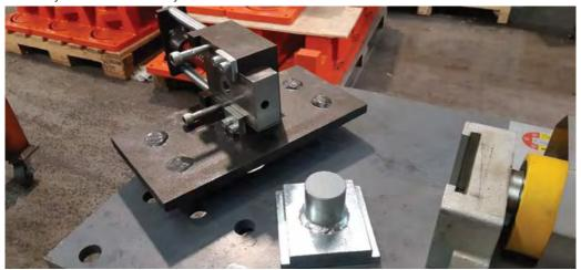
Use the four mounting holes closest to Hydraulic ram as shown. Make sure all 4 mounting nuts are fastened up tight.
