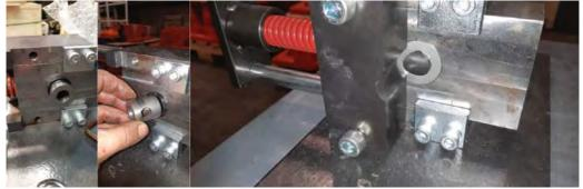
There is a grub screw on the front face of the punch holder/sliding block. Make sure the punch is securely mounted all the way in (no gap between the sliding block face and the punch). Use a plastic or similar soft faced hammer to secure these in place if needed and do up the grub screw on the end face of the sliding block.
