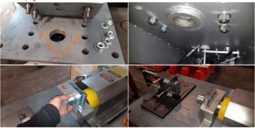
Fit Ram spigot as shown. Do not use any other pushing device on the end of the ram with this cropping attachment or damage to tool or possible injury may occur. The Spigot is designed so the rams tooling chuck will reach the base of attachment before tooling reaches end of stroke (avoiding damage).
