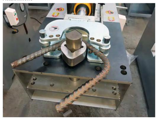
The Rebar Bending Attachment is designed primarily for bending rebar and round mild steel bar up to 32mm diameter. It may be used for bending other material such as mild steel square bar, hexagonal bar, flat bar. It could also be used for straightening bar.
