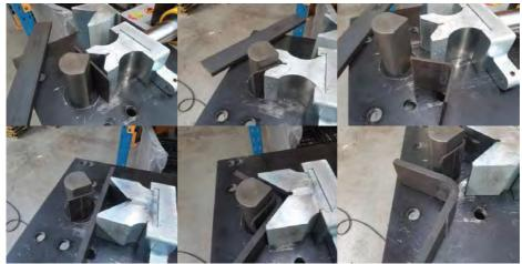
The other option is to heat the part before bending. Spring steels and Tool steels must be bent hot. These cannot be bent cold even in their soft or annealed condition. Stainless steel is less ductile than mild steel and can fracture if bent cold. Extreme care must be taken as
