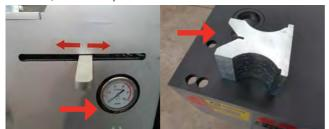
Bending short parts can pose a hazard. Parts can be flipped out of the Bending Anvil if there is not sufficient tail to locate it. Both ends of the bend should be at least 10mm longer then the vee shape in the Bending Anvil.
