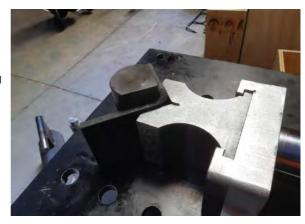
• To bend a piece of steel in the ProBender, Insert mandrill in the large centre hole in the machine as shown. Slide the Bending anvil onto the ram.
