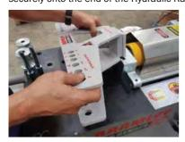
2 Remove the Bending Mandrel (if fitted). Fit the front Former Mount Bracket inside the end of the machine as shown.
