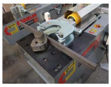
Other possibilities for example, if you need to put a hoop or very large radius in a piece of bar. You can achieve this by pressing a small bend, then moving it along 20mm and repeating.
