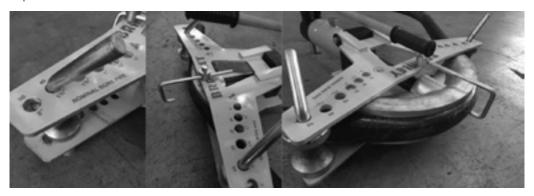
If over time the ram fails to fully extend, or ram seems slow to move, check the level of hydraulic oil in the reservoir with the unit horizontal and the ram fully retracted, open the filler cap. The oil should be covering the cylinder inside unit. The hydraulic unit may need topping up with 32 grade hydraulic oil. (Fluid can be lost if filler cap is not nipped up after use and unit transported or tipped up in this state).
