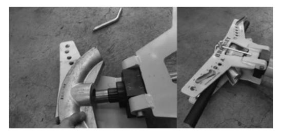
Close the hydraulic valve and using either the fast or slow pistons pump the main ram and former against the pipe and bobbins. Before bend commences, check bend is in desired place. Repositioning is easy up until material bend is started. Bend material until desired angle is achieved. The stop can be set for multiple bends of the same angle. Note there is some bend back when ram is retracted so a slight over bend may be required.
