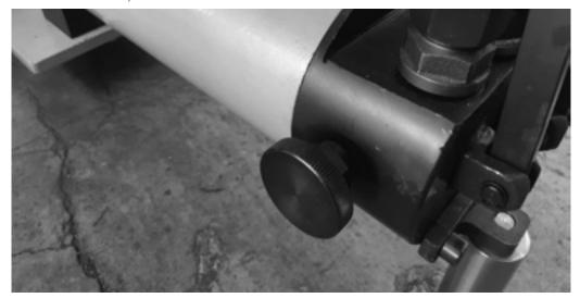
Open the top frame and fit the correct former for the pipe being bent. Fit the pipe being bent and close top frame. Fit the Bobbin and Bobbin pins into the corresponding holes for this size former (if  $1 \frac{1}{2}$ " former fitted the Bobbin and Bobbin pins must be fitted to the  $1 \frac{1}{2}$ " hole).
