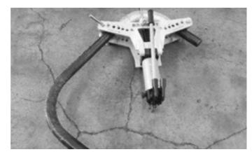
Before using the machine (pumping either pistons or retracting ram) open bleed/filler cap a turn to allow air to escape or enter the hydraulic unit. If the unit is pumped while filler/bleed cap is done up, the unit will simply stop working until you open this.
