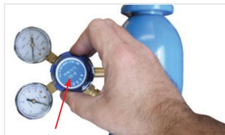
(6) Carefully open the valve of the gas cylinder, set the flow to 6-10 l/min
