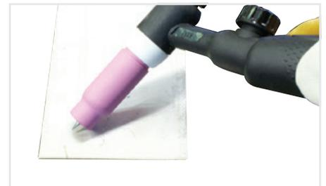
(3) Lay the outside edge of the Gas Cup on the work piece with the Tungsten Electrode 1- 2mm from the work piece.
