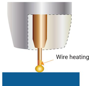
The wire cannot support all the current flow, resistance builds up and the wire becomes hot and weak and begins to melt
