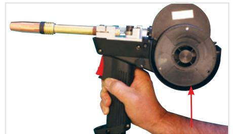
(8) Place a spool of wire onto the Spool holder. Note: the spool retaining nut is Left Hand thread, turn it clockwise to undo it
