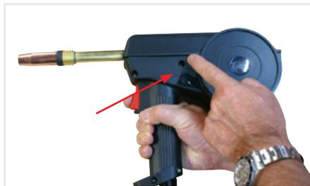
(7) Push the cover release button to unlock the wire feed / spool cover
