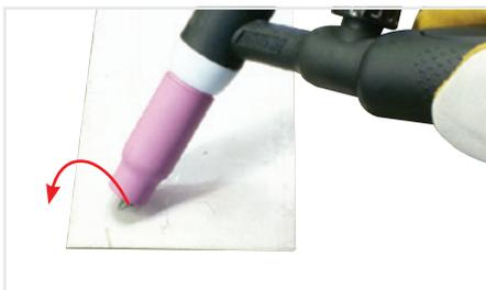
(4) With a small movement rotate the Gas Cup forward so that the Tungsten Electrode touches the work piece.
