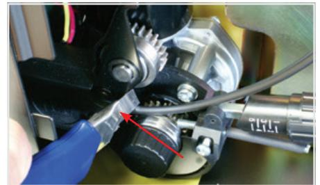
(15) Cut the extended Polymide liner with a sharp Stanley knife just in front of the drive roller
