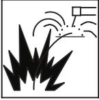
**Fire hazard.** Welding/cutting on closed containers, such as tanks, drums, or pipes, can cause them to explode. Flying sparks from the welding/cutting arc, hot work piece, and hot equipment can cause fires and burns. Accidental contact of electrode to metal objects can cause sparks, explosion, overheating, or fire. Check and be sure the area is safe before doing any welding/cutting.
