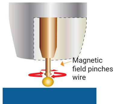
The current flow creates a magnetic field that begins to pinch the melting wire forming it into droplet
