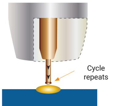
The wire feed speed overcomes the heat of the arc and the wire again approaches the work to short circuit and repeat the cycle.
