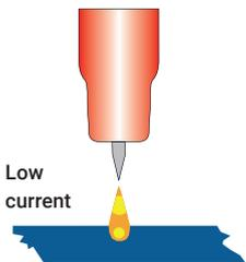
The intensity of the arc is proportional to the current that flows from the tungsten. The welder regulates the welding current to adjust the power of the arc. Typically thin material requires a less powerful arc with less heat to melt the material so less current (amps) is required, thicker material requires a more powerful arc with more heat so more current (amps) are necessary to melt the material.
