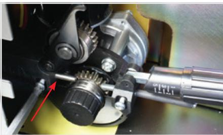
(10) Loosen the inlet guide tube retaining screw.
