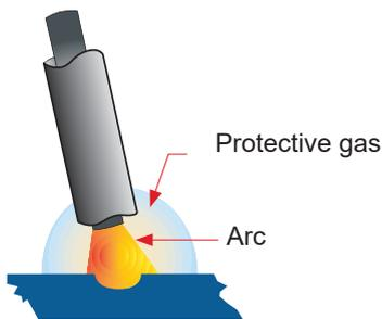
The Metal Wire Core works as conductor of the current that maintains the arc. The core wire melts and is deposited into the welding pool.
