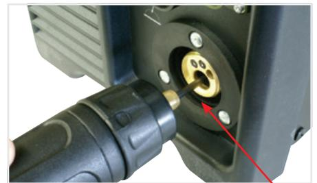
(12) Carefully feed the Polymide liner into the inlet guide tube hole of the torch Euro receptacle
