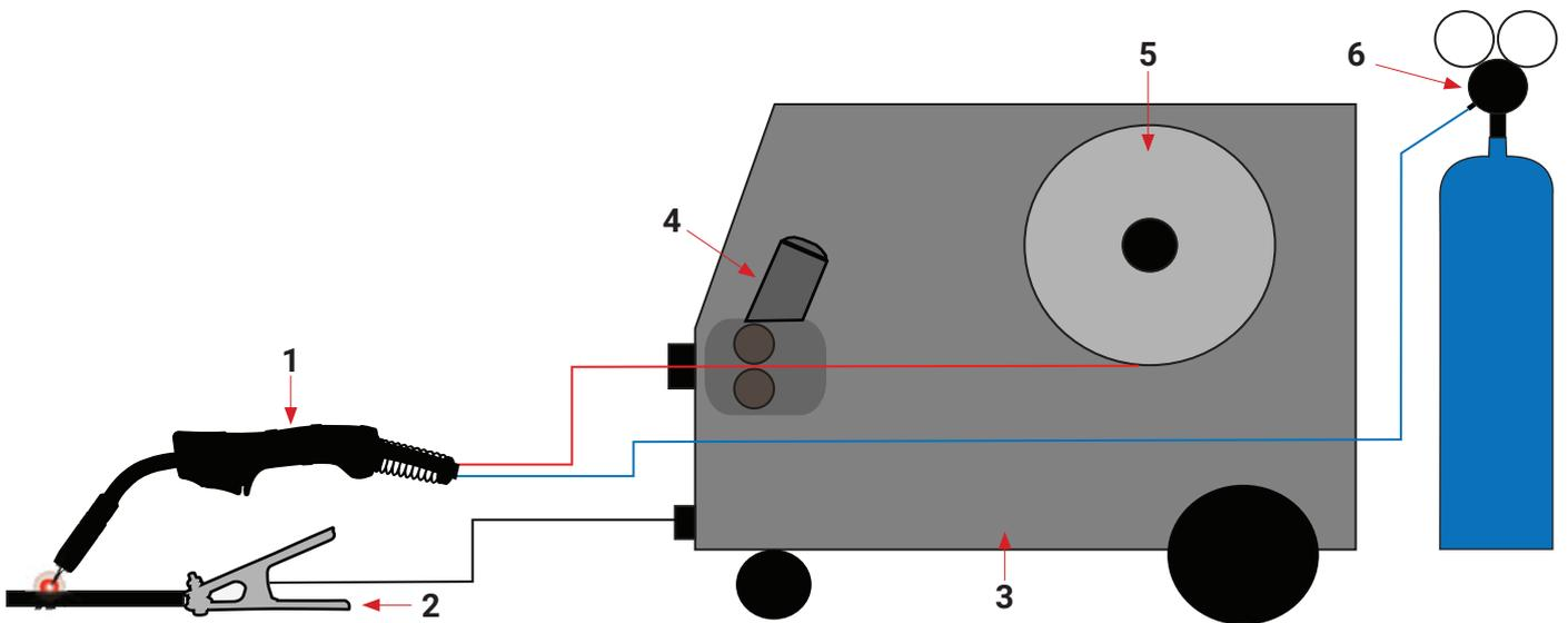
1. MIG Torch - 2. Work Piece - 3. Power Source - 4. Wire Feeder - 5. Wire Spool - 6. Gas
