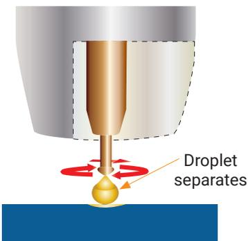
The pinch causes the forming droplet to separate and fall towards the now creating weld pool.
