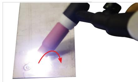
(5) Now rotate the Gas Cup in the reverse direction to lift the Tungsten electrode from the work piece to create the arc.
