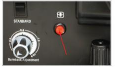
(12) Press and hold the inch wire button to feed the wire down the torch cable through to the torch head.
