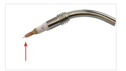
**(12)** Fit the correct size contact tip over the wire and fasten tightly into the tip holder.
