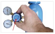
(6) Carefully open the value of the gas cylinder, set the flow to 6-10  $\ensuremath{\mathsf{I/min}}$
