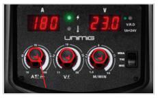
$({\bf 7})$  Set the welding current using the amperage control dial.
