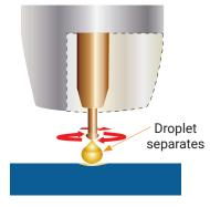
The pinch causes the forming droplet to separate and fall towards the now creating weld pool.
