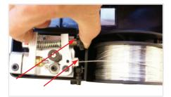
(9) Carefully feed the wire through the inlet guide tube onto the drive roller through into the outlet guide tube. Squeezing the tension arm adjustment knob to release the pressure of the tension arm will allow the wire to be guided through the drive roller easily
