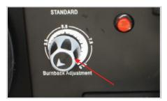
(17) Adjust the burn back control to prevent the wire sticking in the weld pool. Burn back control is located above the wire feed motor
