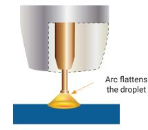
An arc is created at the separation of the droplet and the heat and force of the arc flattens out the droplet into the weld pool. The heat of the arc melts the end of the wire slightly as it feeds towards the base metal
