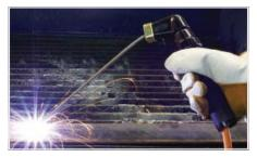
(5) Strike the electrode against the work-piece to create an arc and hold the electrode steady to maintain the arc.
