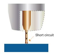
The wire approaches the work piece and touches the work creating a short circuit between the wire and the base metal, because there is no space between the wire and the base metal there is no arc and current flows through the wire.
