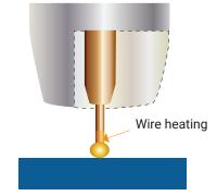
The wire cannot support all the current flow, resistance builds up and the wire becomes hot and weak and begins to melt
