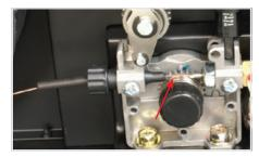
(8) Feed wire over the drive roller into the outlet guide tube, Push the wire through approx 150mm.
