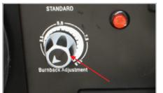
(16) Adjust the burn back control to prevent the wire sticking in the weld pool. Burn back control is located above the wire feed motor
