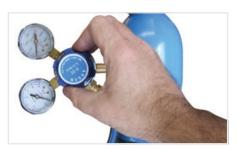
$({\bf 15})$  Carefully open the valve of the gas cylinder, set the flow to 8-12 L/min
