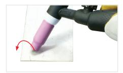
(4) With a small movement rotate the Gas Cup forward so that the Tungsten Electrode touches the work piece.
