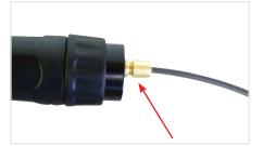
(8) Push the liner firmly into the torch lead and tighten the liner retaining nut
