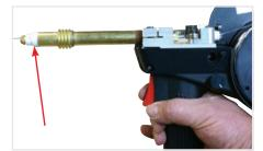
(12) Remove the gas nozzle and contact tip. Pull the trigger to drive the wire through the neck until it exits the contact tip holder
