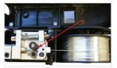
(10) Check to make sure that the wire passes cleanly through the drive roller into the outlet guide tube.
