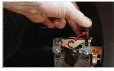
(9) Close down the top roller bracket and clip the pressure arm into place. Apply a medium amount of pressure to the drive roller
