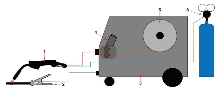
1. MIG Torch - 2. Work Piece - 3. Power Source - 4. Wire Feeder - 5. Wire Spool - 6. Gas
