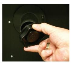
(1) Remove the spool retaining nut.
