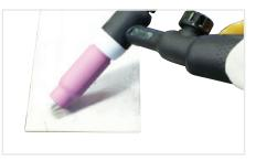
(3) Lay the outside edge of the Gas Cup on the work piece with the Tungsten Electrode 1- 2mm from the work piece.
