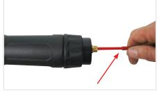
(3) Carefully pull out and completely remove the liner
