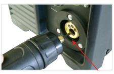
(12) Carefully feed the Polymide liner into the inlet guide tube hole of the torch Euro receptacle
