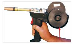
(8) Place a spool of wire onto the Spool holder. Note: the spool retaining nut is Left Hand thread, turn it clockwise to undo it
