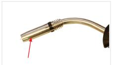
**(17)** Fit the remaining front end parts to the torch neck ready for welding.
