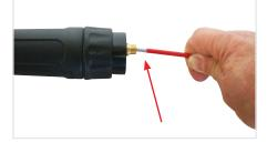
(5) Carefully feed in the new liner down the torch lead all the way to exit the torch neck.
