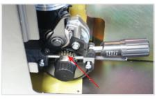
(9) Install a U groove drive roller of the correct size for the diameter wire being used.
