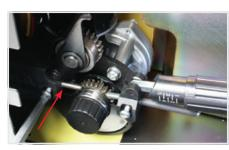
(10) Loosen the inlet guide tube retaining screw.
