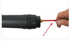
$\ensuremath{\textbf{(3)}}$  Carefully pull out and completely remove the liner
