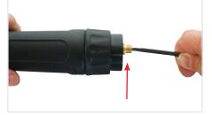
(5) Carefully feed in the new liner in short forward movements down the torch lead all the way to exit the torch neck. Be careful not to kink the liner
