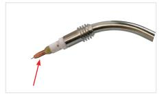
(16) Fit an Aluminium contact tip of the correct size to match the wire diameter being used
