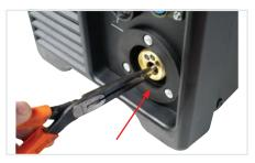
(11) Remove the inlet guide tube using long nose pliers.
