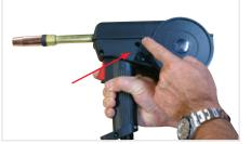
(7) Push the cover release button to unlock the wire feed /spool cover
