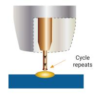
The wire feed speed overcomes the heat of the arc and the wire again approaches the work to short circuit and repeat the cycle.
