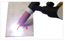
(5) Now rotate the Gas Cup in the reverse direction to lift the Tungsten electrode from the work piece to create the arc.
