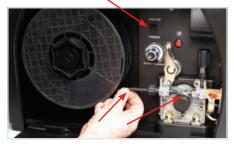
(7) Place wire onto spool holder - (spool retaining nut is left hand thread ) Feed the wire through the inlet guide tube into the drive roller.
