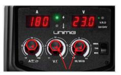
**(15)** Set welding parameters using the voltage and wire feed controls.
