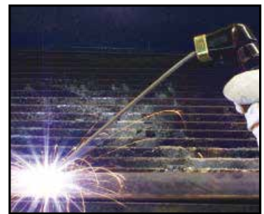
(5) Strike the electrode against the workpiece to create an arc and hold the electrode steady to maintain the arc.
