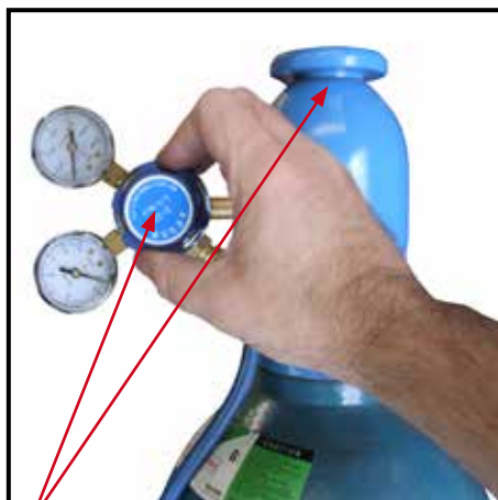
(4) Carefully open the valve of the gas cylinder, set the flow to 8-10 l/min
