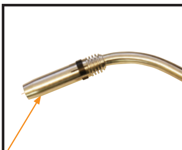
(13) Fit the gas nozzle to the torch head.
