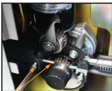
(10) Loosen the inlet guide tube retaining screw.
