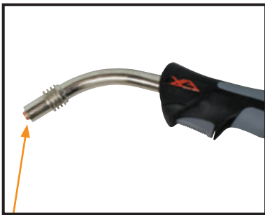
(1) Remove mig torch front end parts
