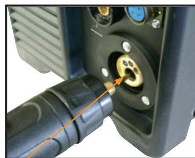
(12) Carefully feed the Polymide liner into the inlet guide tube hole of the torch euro receptacle
