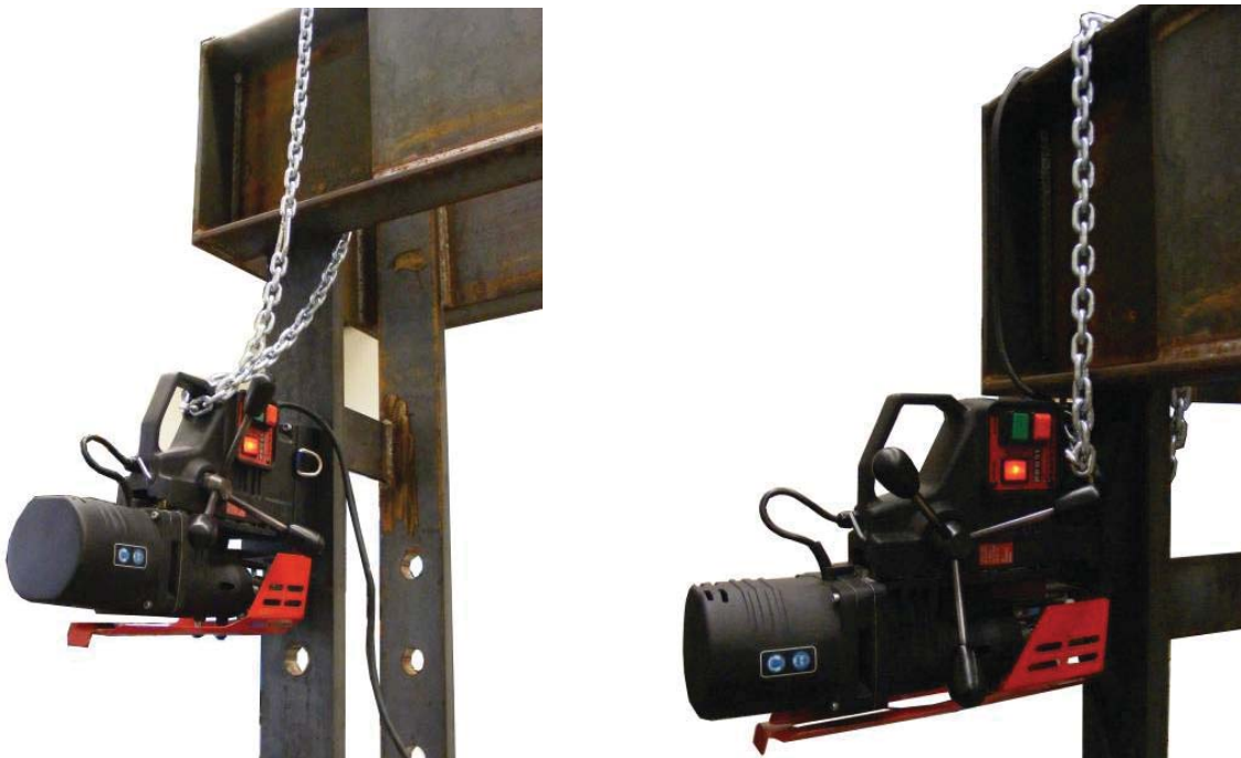
An example of a safety chain/strap use.
