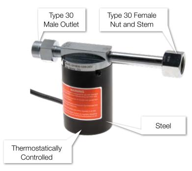
The Type 30 model gas heater is attached directly in between the cylinder and the regulator (or connection lead on manifolds) warming the gas prior to entering the regulator.
