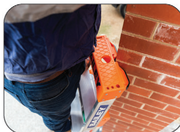
Outside corner leaning
