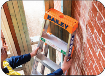
Inside corner leaning
