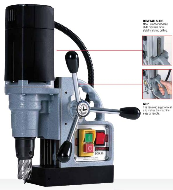
The ECO.30 is light and super fast. Weighing in at only 8.5kg, the ECO.30 packs a punch. The lightest drilling machine on the mearket, it will drill a 14mm hole through 12mm steel plate in only 5.9 seconds.
