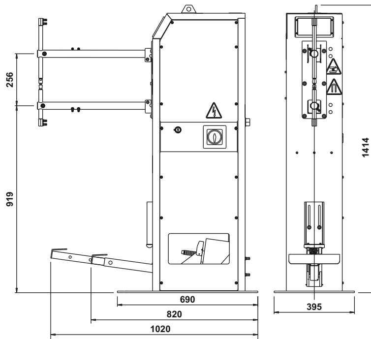
PUNTATRICI PNEUMATICHE - AIR OPERATED SPOT WELDERS - SOUDEUSES PAR POINTS PNEUMATIQUES
