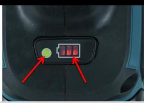
Automatic Torque Drive indicator and Battery Fuel Gauge highlighted with LED's
