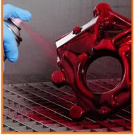
Locating critical defects with Red Dye Penetrant
