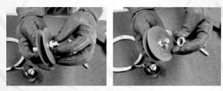
Step 2: Assemble the outlet to what will be your trailing baffle. Like with the forwaqrd baffle, insert the threaded portion of the gas outlet through the centre hole of the baffle and secure with the nut.
