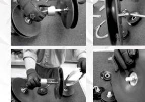
Step 5: Connect the trailing baffle to the trailing connecting arm.
