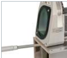
Precise adjustment of the electrode's stick-out.
