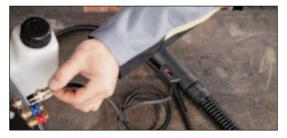
8. Connect the flow control cable to the cooling unit.
