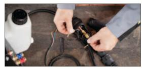
2. Disassemble end of the trigger cable.
