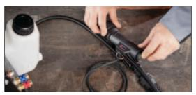
6. Lead out the flow control cable through the control cable outlet out of the housing.
