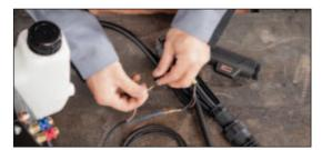
**3.** Connect the trigger cable to the flow control
