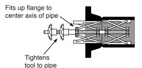
Two independently operated internal mandrels align flange to pipe even if internal dimensions differ.
