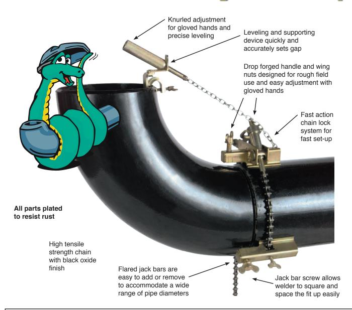
The Clamp Champ is built for the welder who takes pride in doing his job right the first time. Constructed for years of trouble free job site use, the versatile Clamp Champ makes pipe fit-up simple and accurate – without the need of a helper. The Clamp Champ is similar to a pipe vise with fast, easy set up and solid chain engagement.
