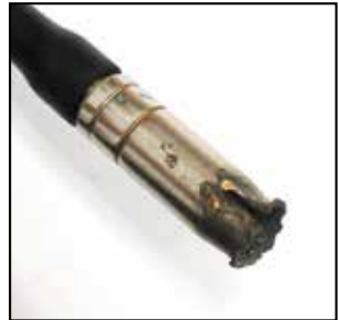
Build up of spatter can cause damage to nozzle and tip
