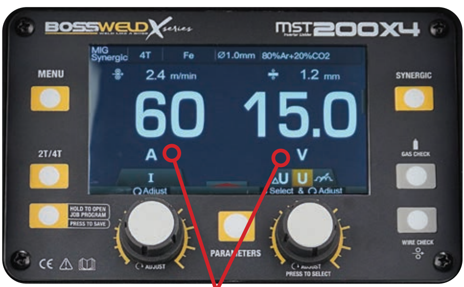
Amperage and Voltage display
