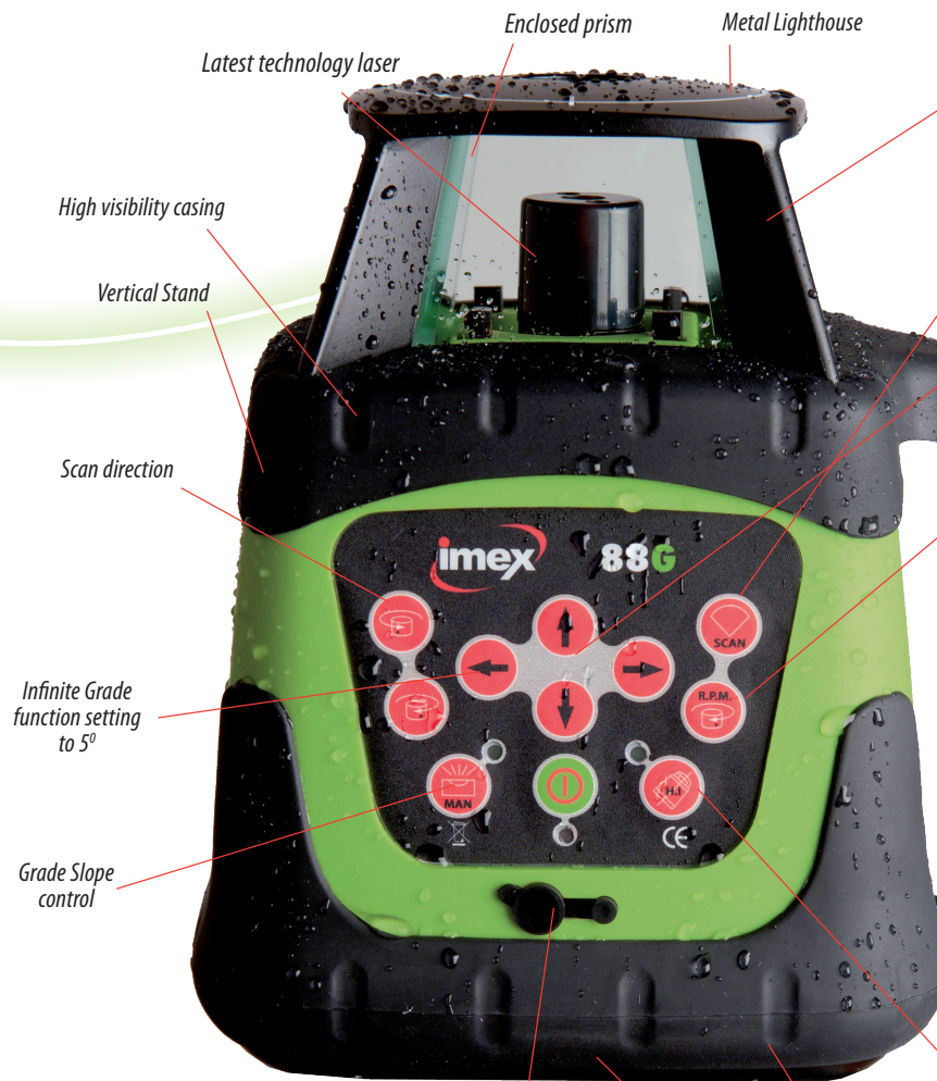
Magnetic head Rechargeable battery Reinforced base Plumb spot
