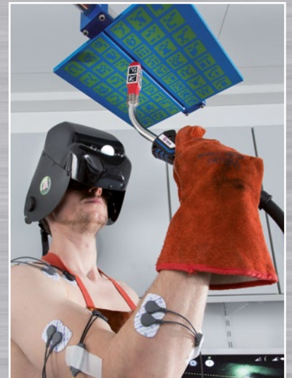
MB EVO PRO 36 in welding position PE (overhead welding).
