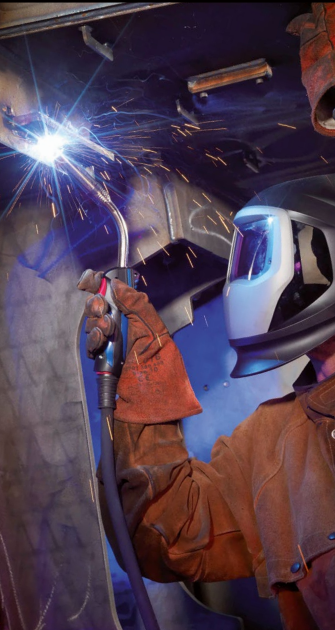
MB EVO PRO 36 in welding position PA (horizontal welding of butt and fillet welds).
