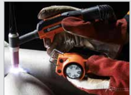
R 10 hand remote offers convenient current control at a distance, for both TIG and MMA process.
