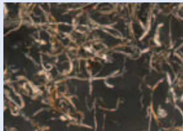
Long chips generated with the POLIFAN®-STRONG-FREEZE. No blue colouration due to low thermal loads.
