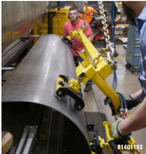
Press Brake Loading
