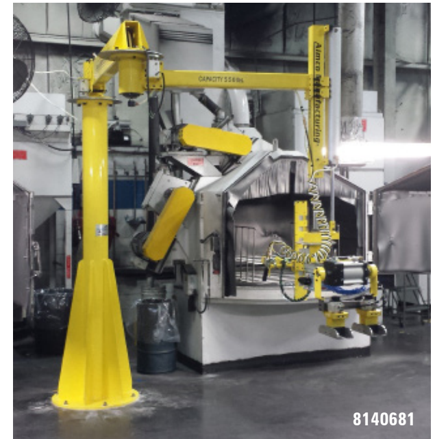
Bead Blasting Load Operation
