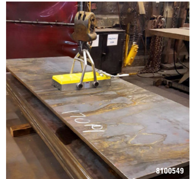
Heavy Sheet Handling with MLAY1000x12
