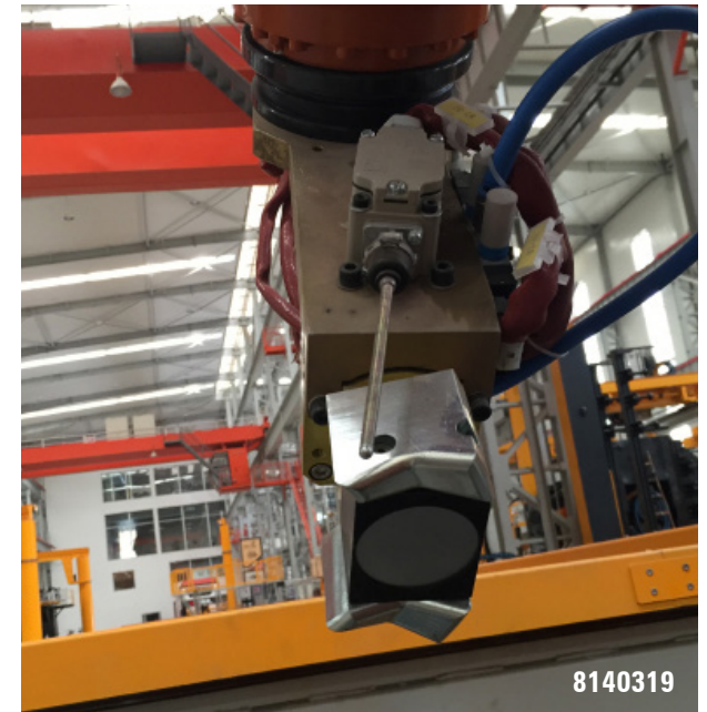
Custom Locating Pole Shoes for U Pipe
