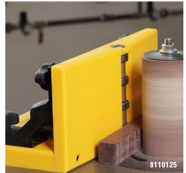
Sanding & Facing with Resaw Guide
