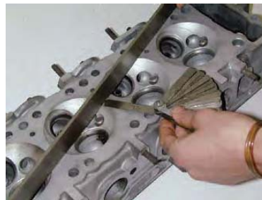
Straight Edge being used to check flatness of an engine block.
