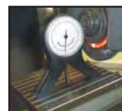
Check table alignment in the horizontal plane
