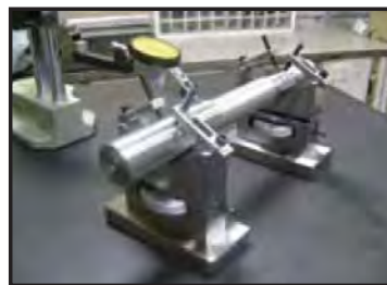
Adjustable Vee Block being used to check concentricity of different diameters on a stepped rod
