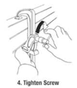
1. Loosen Screw 2. Push in Jaw Base 3. Slide Jaw Up or Down 4. Tighten Screw
