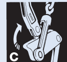
As the chain tension is released, the handle will remain almost in the same position.
